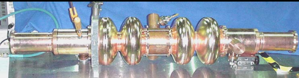
1.5 GHz model of 'superstructure' cavity with coaxial HOM couplers
